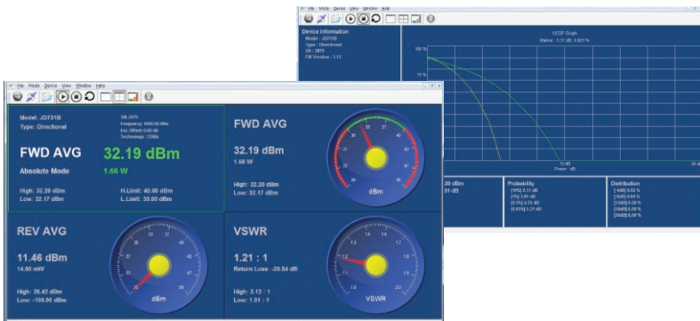
Power meter measurements shown on a PC
