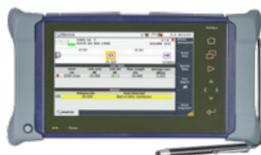
Two-slot handheld modular platform for testing fiber optic networks
